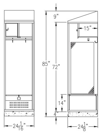
PLEASE BE ADVISED: Lockers Are Square And Measured Based On Square Walls. If Walls Are Not Square, Adjustments To Bases Will Need To Be Made At The Expense Of The Customer To Make Allowances For The Locker Sizes As Specified In The Shop Drawings.
