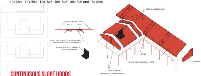
Continuous Slope Hoods fit on top of flat top lockers. They can be used on new lockers, or on a retrofit basis. All hoods are furnished in 72" lengths and must be cut to length during installation. Intermediate splices, ends and rear supports (2 per hood) complete the installation, and must be ordered separately.
