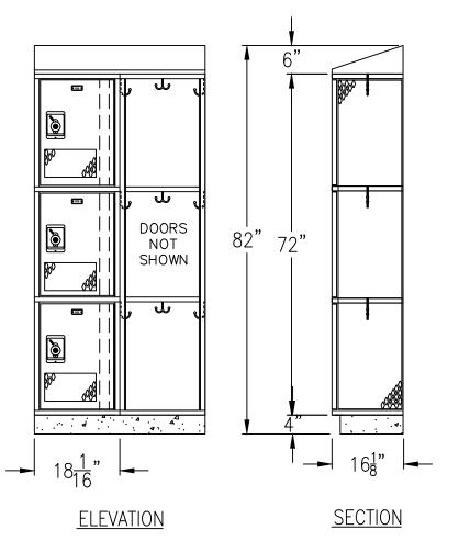
PLEASE BE ADVISED: Lockers Are Square And Measured Based On Square Walls. If Walls Are Not Square, Adjustments To Bases Will Need To Be Made At The Expense Of The Customer To Make Allowances For The Locker Sizes As Specified In The Shop Drawings.
