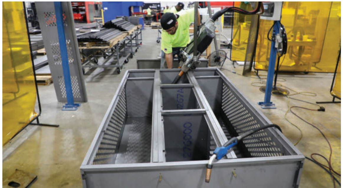
An employee positions a resistance spot welding head to join a locker frame member. Stations also incorporate gas metal arc welding. Note the C-frame return flange around the perimeter. These extra bends add strength to the assembly.
