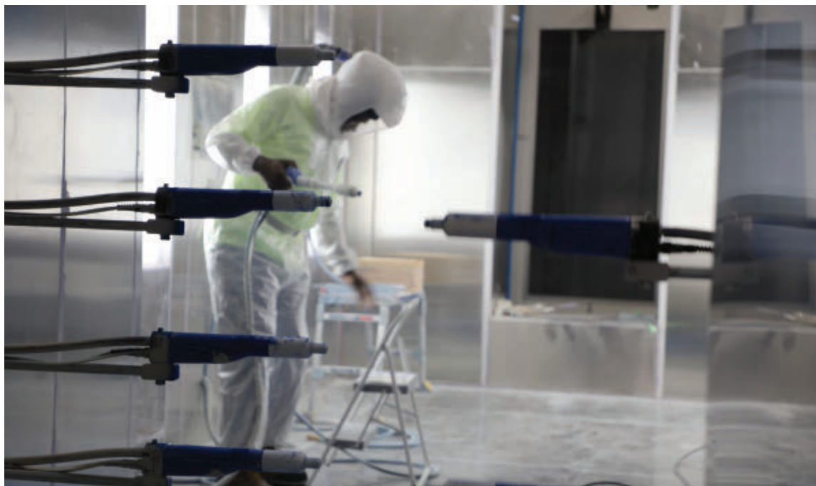
A powder coating technician, standing behind a row of mechanized coating guns, preps for a job.
